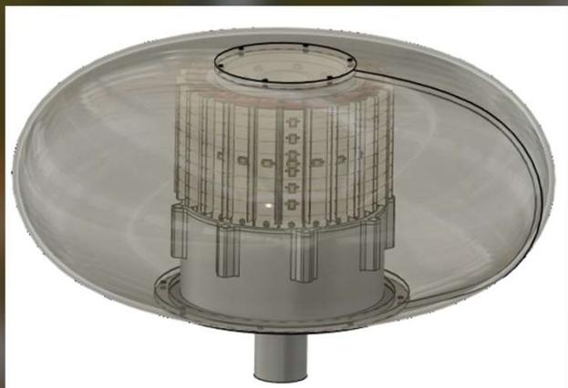
*Radome composite fibre de verre/mousse ( $\Phi = 56 \text{ cm}$ ,  $h = 25 \text{ cm}$ )*
